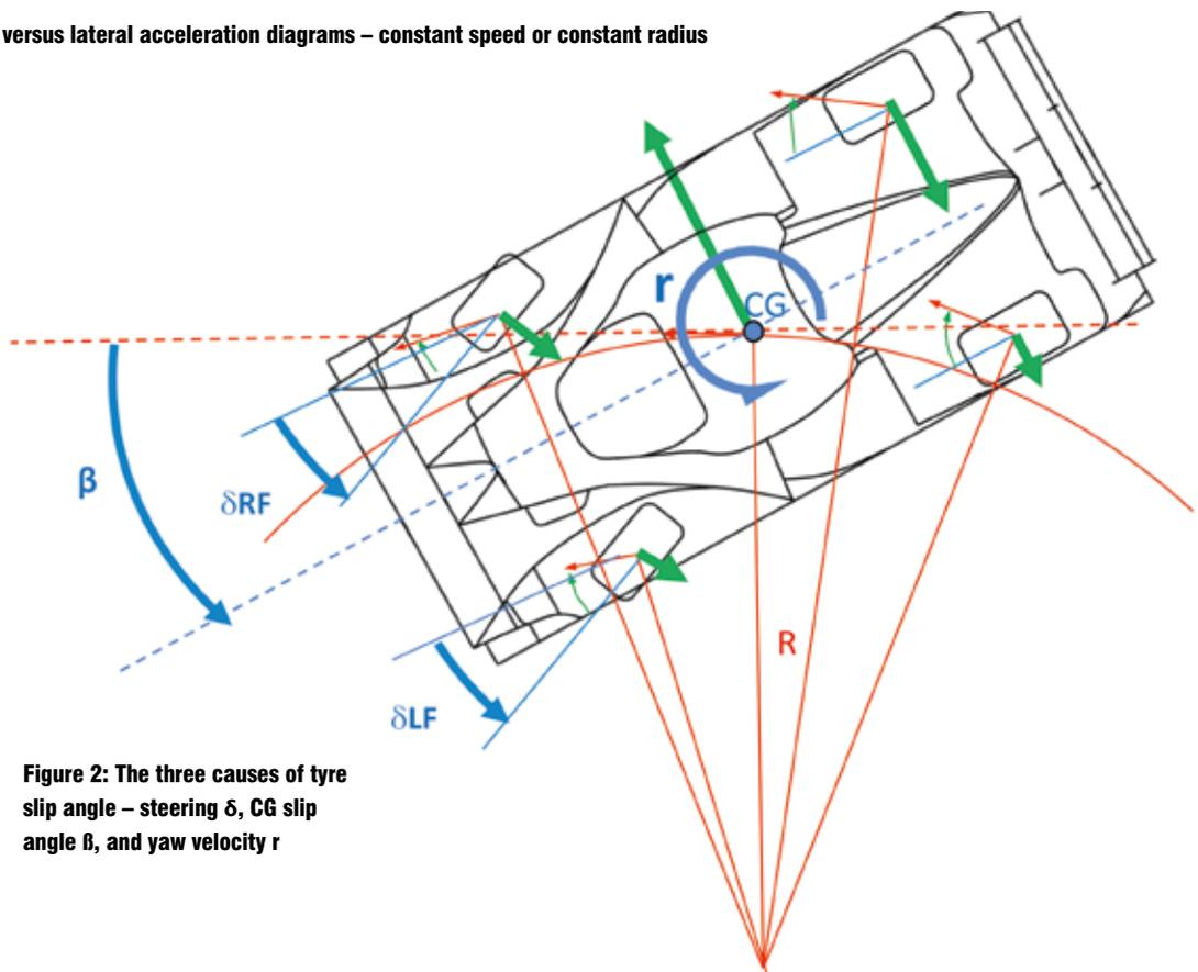
**Figure 2: The three causes of tyre slip angle – steering  $\delta$ , CG slip angle  $\beta$ , and yaw velocity  $r$**
